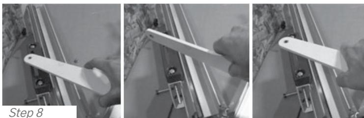
**STEP 8:** Flip the lift-arm over and reinstall the shoulder bolt with its jam-nut.
