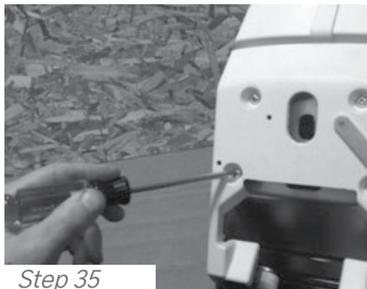
**STEP 35:** Use a #2 Phillips screwdriver to remove the lower safety switch bumper from the Rave unit. It has four screws.
