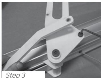
**STEP 3:** Catch the link and set it aside. Be careful not to damage the paint.
