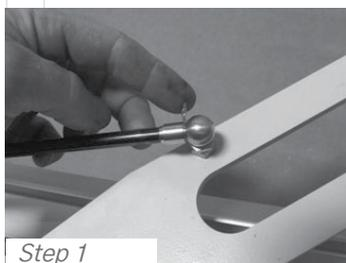
To remove the ball mounts, remove the wire retainer clips that hold them on. Pull the ball-ends straight-up to remove.
