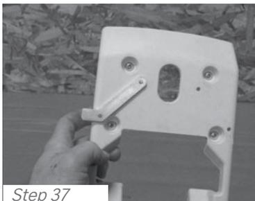
**STEP 37:** Flip the arm to the other side and reinstall it. The necessary holes should already be in the safety bumper.
