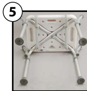
Lay the bench on the floor so that the back of it is facing upward. Place the back tubes through the rear tube guides. Depress the brass push pins and insert the end of the tubes through the front tube guides until the pins engage into the rear tube guide. (The back can be adjusted to a deep or shallow position depending on user preference.) Be sure pins are fully engaged by pulling on the back.
