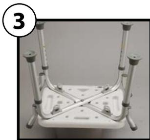
Attach the legs by telescoping the adjustment leg over the leg stem and pushing the push pin in. Be sure to adjust all four legs to the same adjustment holes.
