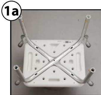
Set the seat on an elevated surface face down and place the leg marked 2 into the diagonal inset on the bottom of the seat. (The #2 on the seat should line up with the #2 label on the tube. Repeat for tube labeled #1 so that tube #2 is under tube #1. Insert #1 screw w/ washer into the center hole and tighten.
