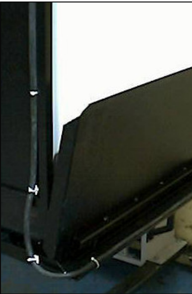
FIG. 14- FASTEN CABLE TO SAFETY PLATE USING STRAPS
