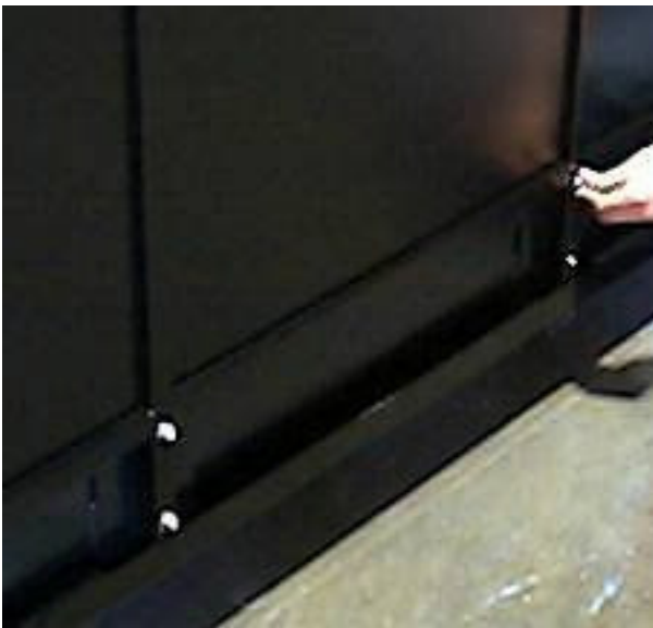
FIG. 6B- BOLT HANDRAIL TO CARRIAGE
