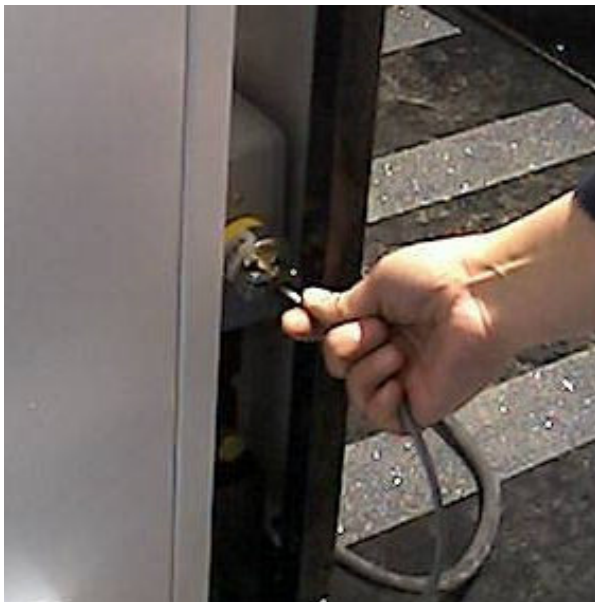
FIG. 2- PLUGGING IN UNDER DECK SAFETY LIMITS
