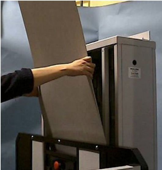
FIG. 3- REMOVE FRONT PANEL
